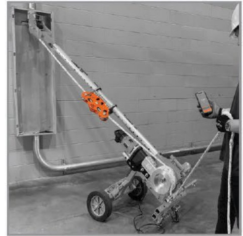
Overhead & Right Angle Pulls
